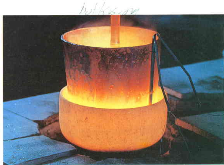
Ultra-purity is a prerequisite for melting superior optical glass. This melting crucible might well be one of the most valuable of its type. It is made of pure platinum.
